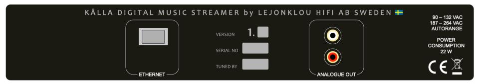
**Start** by connecting an Ethernet cable between the router of your local network and Källa. Make sure **there isn't excessive strain** on Källa's Ethernet port. It's often beneficial to have a network switch (e.g. Netgear GS-108T) in between the router and Källa. We recommend that the Ethernet cables are kept as short as possible, but never shorter than 2.5 m.
