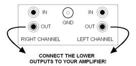
Make sure the connectors are pushed all the way in, but **beware of using excessive force** as you might cause cracks in the circuit board. If connectors are too tight or too loose, the music will suffer.
