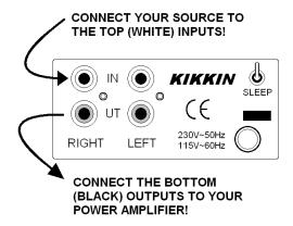
Please note that Kikkin inverts the phase to your power amplifier. Therefore connect the positive output (red) of the power amplifier to the negative (black) loudspeaker terminal, and the negative output to the positive loudspeaker terminal.
