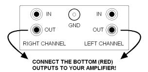
If your turntable has a ground lead, connect it to the large ground screw. Last of all, connect the power cord.
