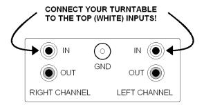
Please note that the colours white and red do not correspond to left and right – the connectors were chosen for best sound quality and black sockets unfortunately proved impossible to order. Now connect a good pair of interconnects from the outputs (red) to a pair of line level inputs on your amplifier as shown below.
