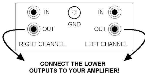
If your turntable has a ground lead, connect it to the large central ground screw.
